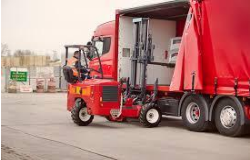
Fig VU2. Safe Un-loading using FLT
