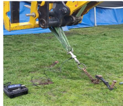
Fig EK 2. Stake pull test
