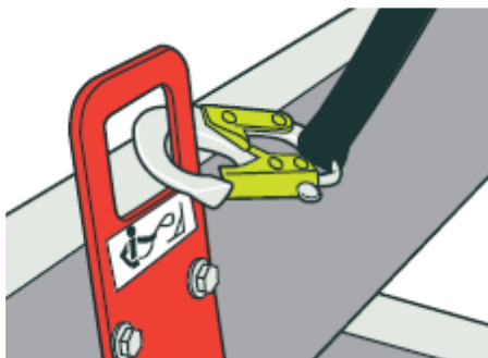
Fig PL5. MEWP anchorage point for operator and IPAF emergency descent location indicator
