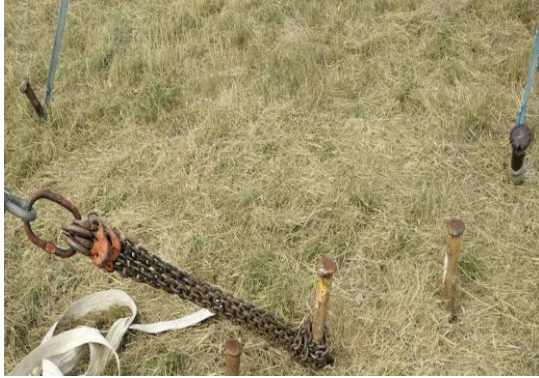
Fig EK 1. Ground Anchors/Stakes
