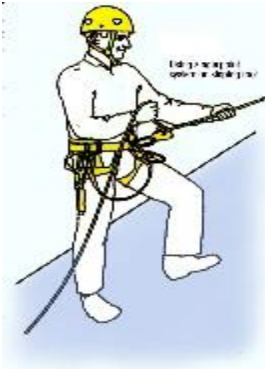
Fig WH1. Worker climbing mast using safety line and ASAP unit
