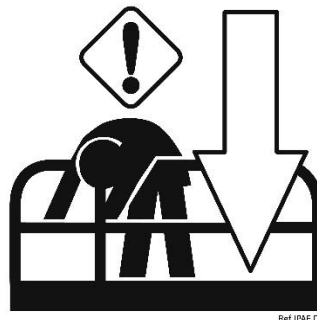
Fig PL5. MEWP anchorage point for operator and IPAF emergency descent location indicator
