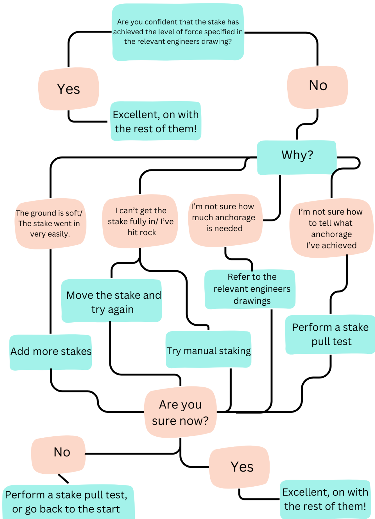
Fig EK7. Process for ensuring integrity of stakes
